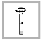
2. Screw an orange colored **DosiCap B** onto the cuvette.
